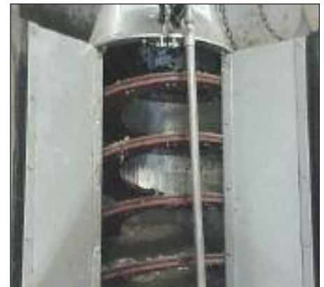
Durable spiral brush keeps the screen clean.
