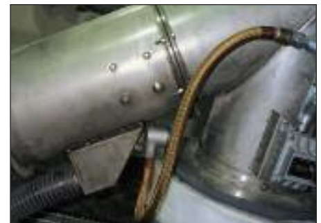
Close-up view of the new drain box with optional explosion-proof wiring.
